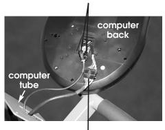
(10) wire connector leads to the motor/magnetic sensor/ AC adapter jack
